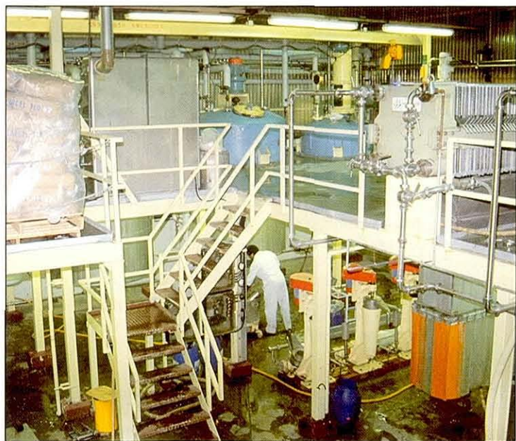
Protein hydrolysate manufacture showing hydrolysis vessels in background
